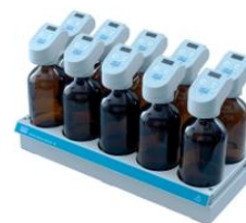
BOD Sensor System 10
